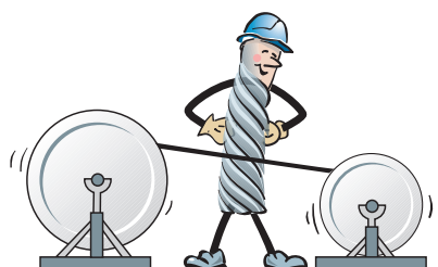
Figure 2-5 - do not create a reverse bend Figure 2-6 - Installing rope under tension, about 10% of the nominal rope pull
